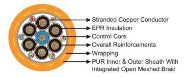
Conductor: Stranded bare copper conductor, Class 5/Class 6 to VDE 0295/IEC 60228.
